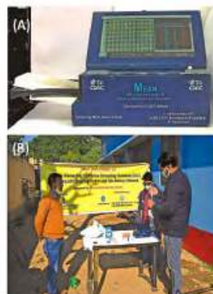
Biosensing prototype device for OPs pesticide detection (A) and Deployment of prototype device at wetlands of Assam (B)
